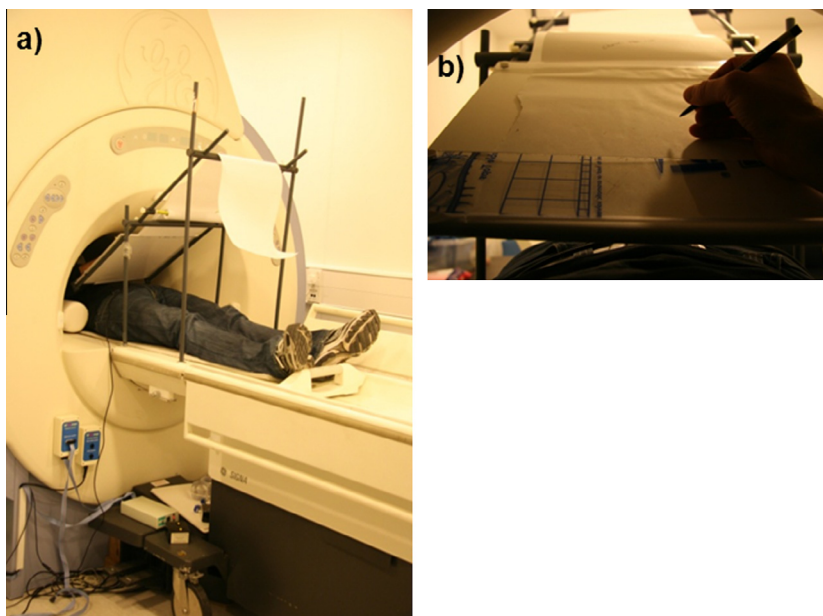
Fig. 1. (a) Experimental set-up showing a participant lying in the 'mock' training scanner. A paper roll, mounted on a specially-constructed writing frame, was advanced manually by the experimenter after each trial. (b) Participant's perspective image taken from inside the bore of the training scanner. The participant's eyes were closed throughout the experiment.
